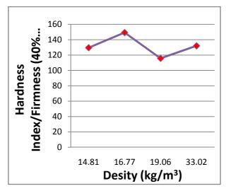
Figure 7: Graph of Hardness Index/Firmness (40% IFD) against Density
